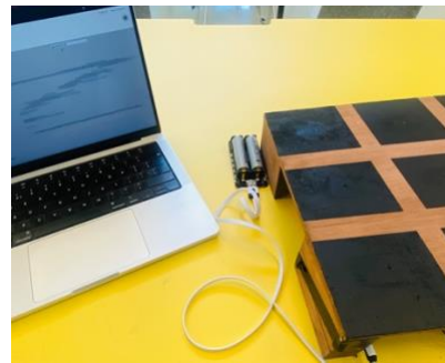
Fig. 4. A DIY touchboard built with conductive paint, wirelessly sending capacitive touch data to a laptop running a particle-based data visualisation.
