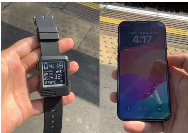
Figure 1 - Comparison between LCD and E-Paper in a sunny environment (iPhone on full brightness).
